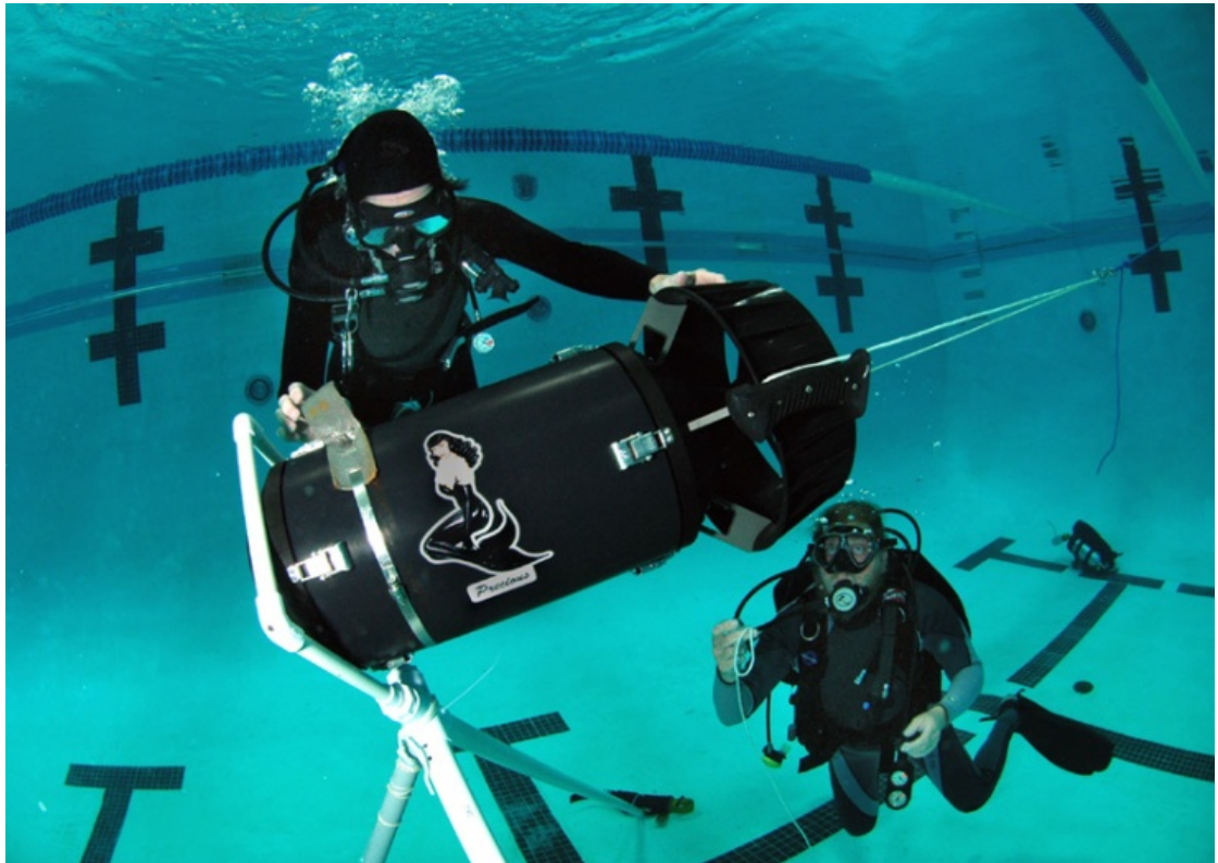
The Gavin Short is loaded into the test stand for thrust testing. Photo by Chuck Weber
