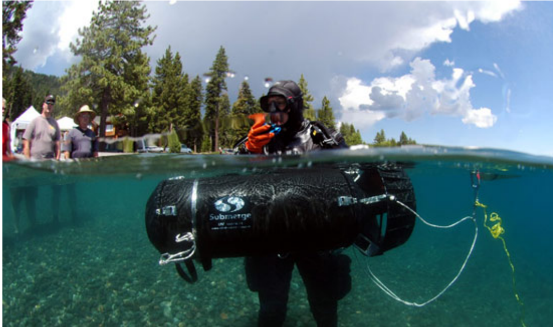
The UV-26 test article. Because the draw was distributed over two battery packs, this model extracted the rated capacity from its battery packs. Photo by Chuck Weber
